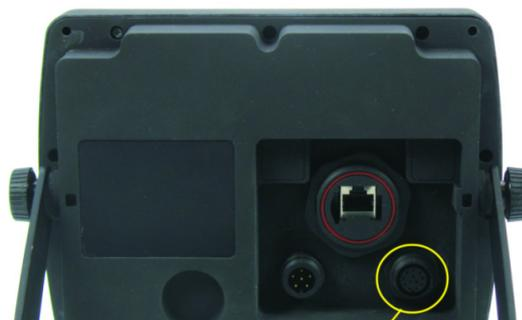
Figure 8-20 Pilot port connection, TR-8000 Display unit (rear)
