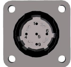
Figure 8-28 AMP 206486-1 Pinout
