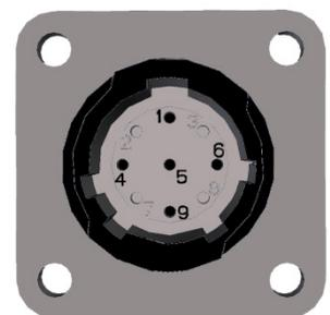
Figure 8-23 AMP 206486-1 (Pilot Socket) pinout
