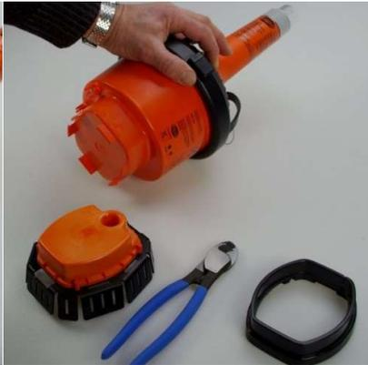
Take a solid grip around the Storage Module and release the unit from the Capsule
