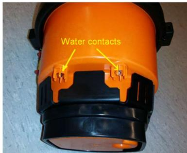
**IMPORTANT;** during the following process, do not get in direct contact with the water activation contacts with wet hands or expose these to water.
