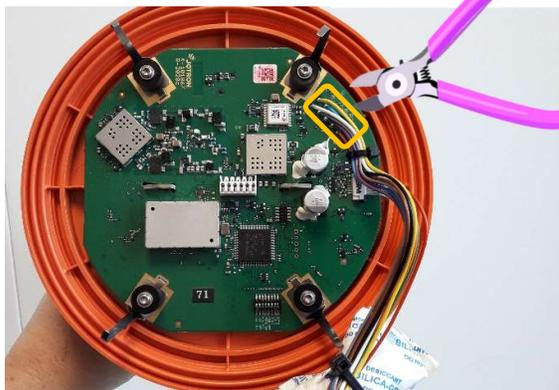
Snip off the battery connection cable close to the circuit board. This renders the electronics unusable.
